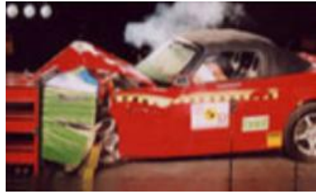
Offset crash test at 64km/hr
